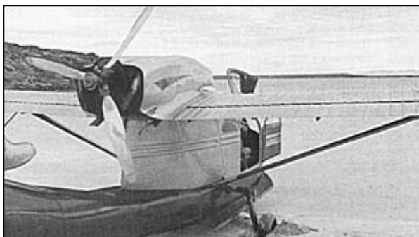
The right gear has rolled into the hole dug for it, waiting for high tide. If the tide were not present, and thus not a factor, more digging would be required.
